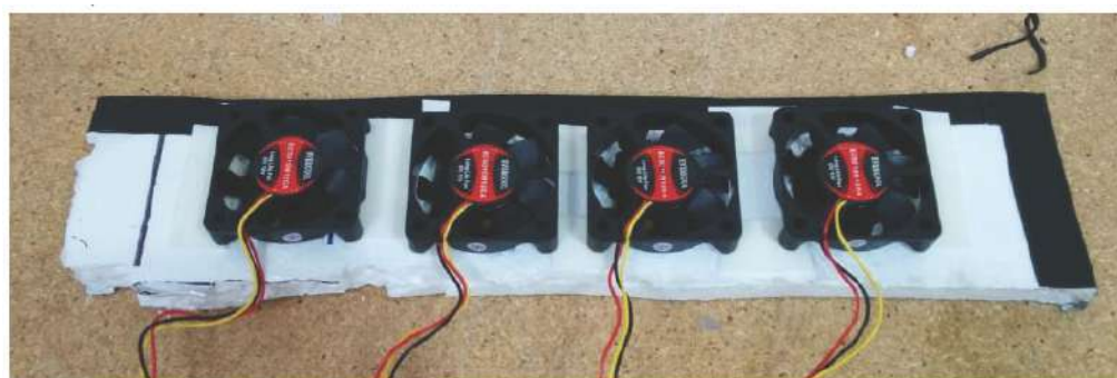
Figure 15. The bank of fans, which sit on top of the open portion of the air distributor as shown in the right image in Fig. 14.
