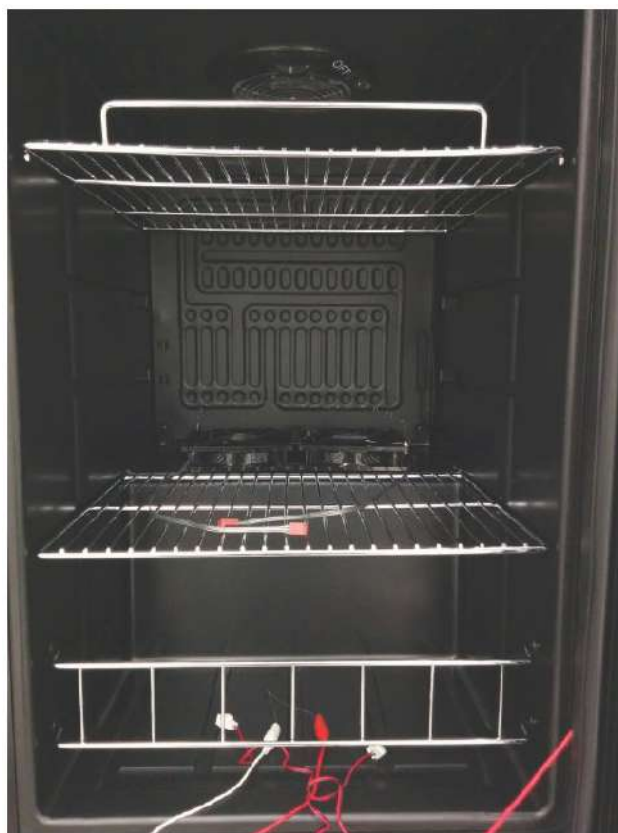
Figure 13. The back of the enclosure showing the cold wall built into the cooler, the two 12 V fans, and (barely visible above the fans) the heating wire.
